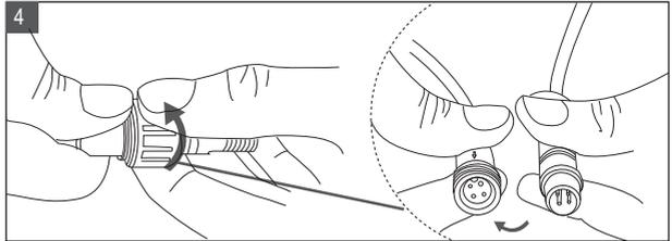
5. Connect the control panel to the spa tub. Fasten and secure the rings to the pipe adapter on the spa tub. (Fig.4) Make sure the rubber O-rings are properly placed on the air pipes.
