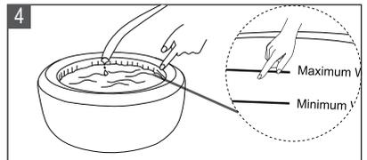
Do not over fill the spa. It is recommended to fill the spa with lukewarm water for quick heating and energy saving.
